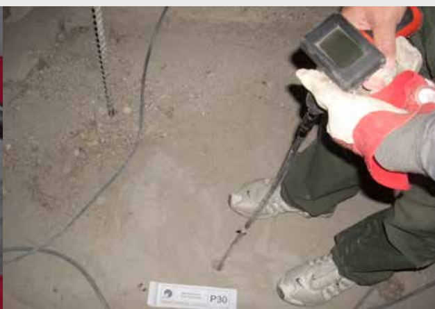
On-site test: Endoscopy
