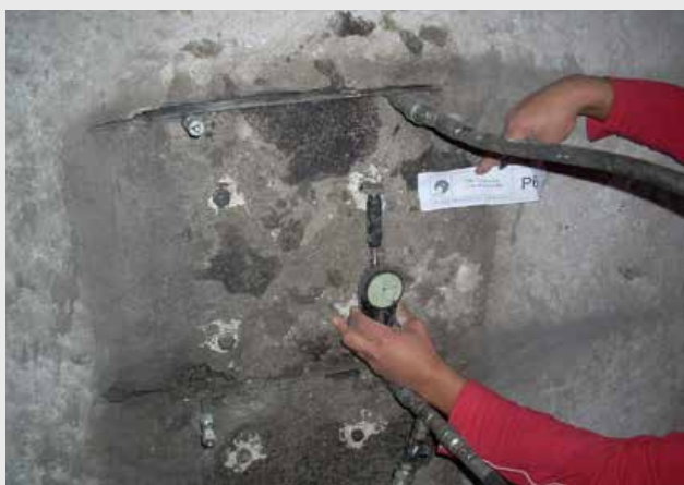
On-site test with Double Flat Jacks
