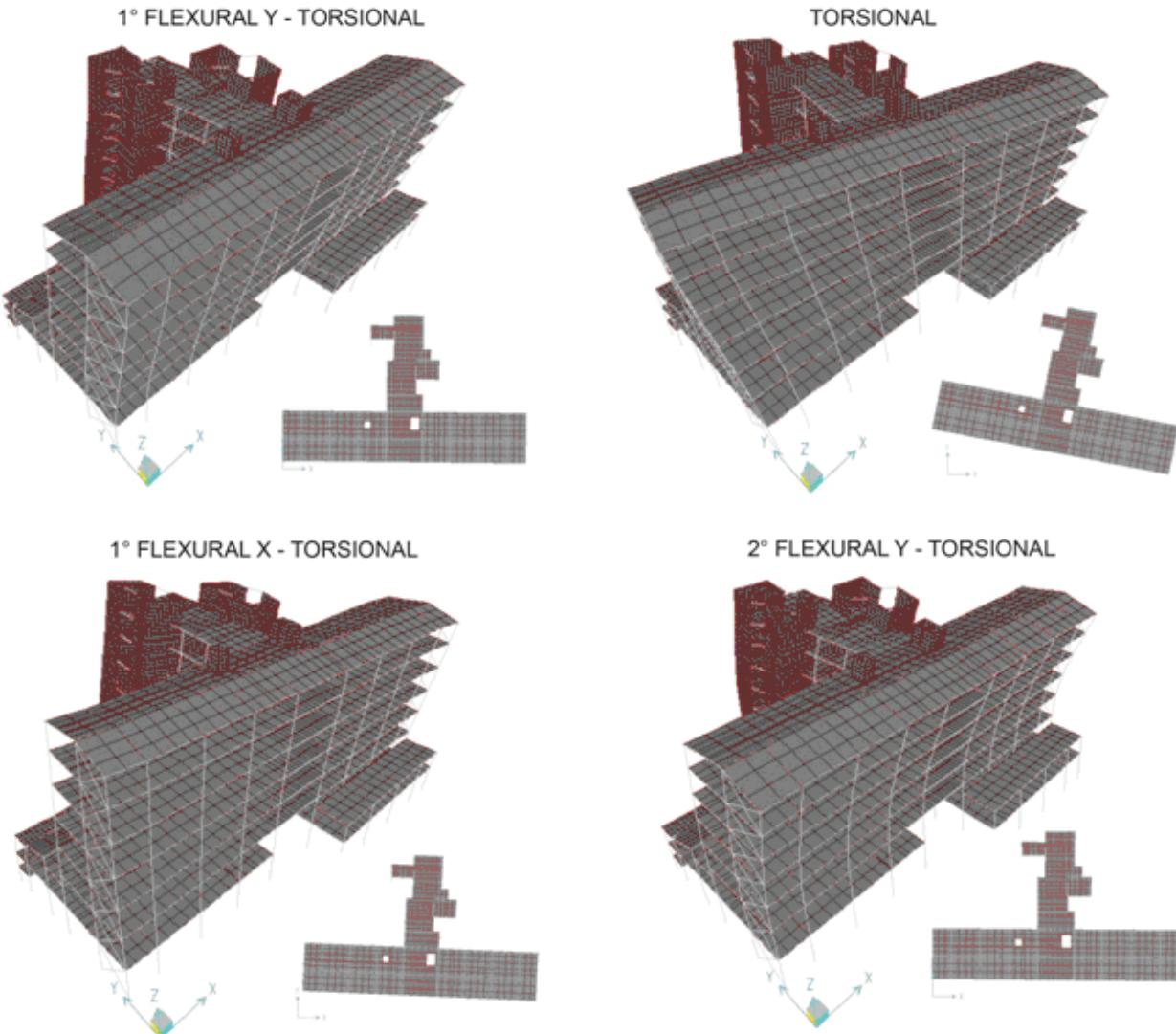
Figure 6. Calibrated mode shapes.
