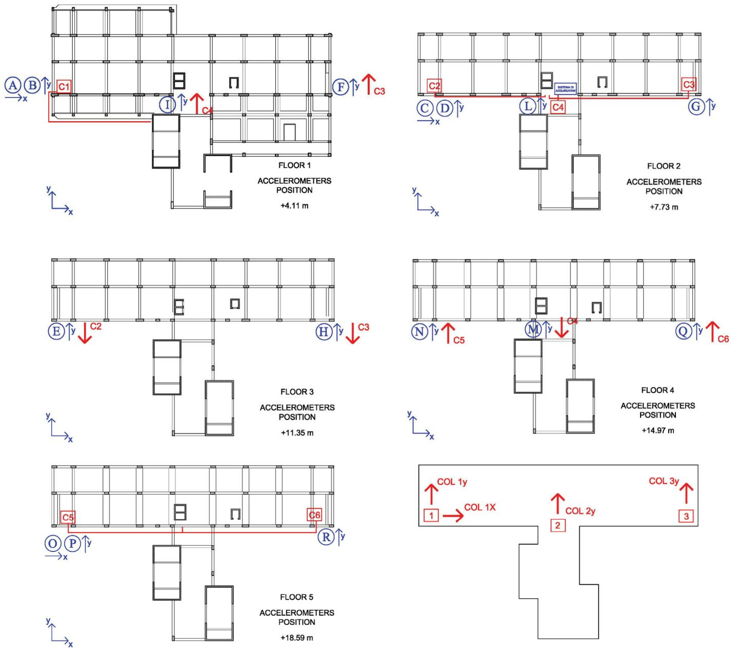
Figure 4. Location of the sensors, at different floors, during environmental vibration test.
