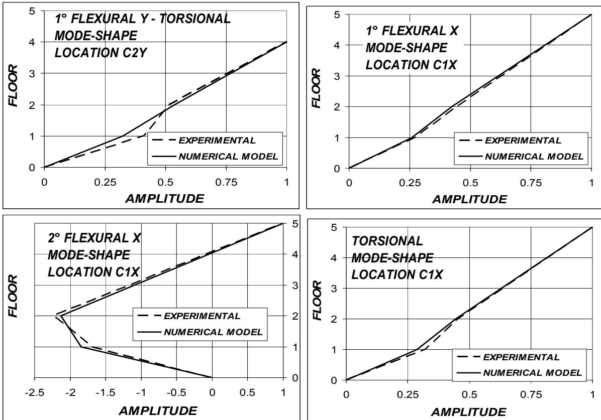
Figure 7. Displacement pattern for experimental and numerical mode shapes.
