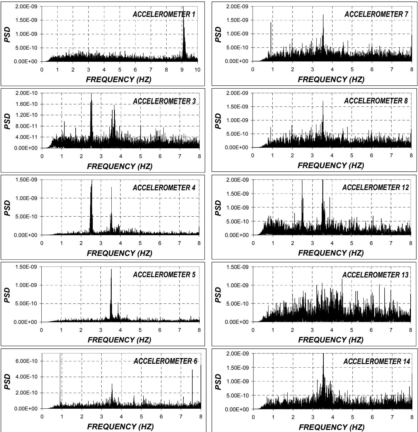
Figure 5. Power spectral density of the accelerometer response.
