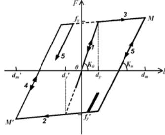
**Figure 4.** The CANNY BL2 material model assumed for steel brace (Li 1996).
