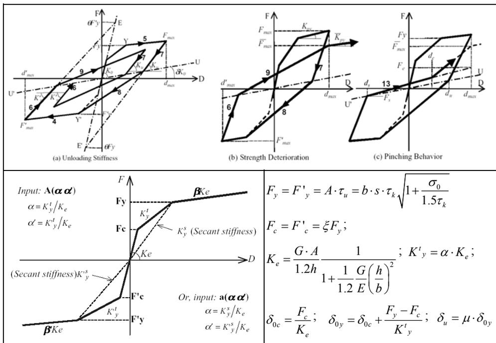
**Figure 3.** The CANNY CA7 material model assumed for masonry (Li, 1996).
