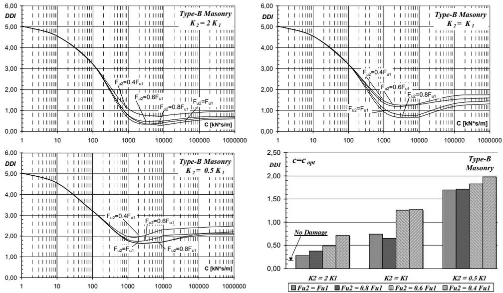
Figure 8. Type-B masonry: values of DDI as a function of viscous constant  $c$  (Calitri earthquake).
