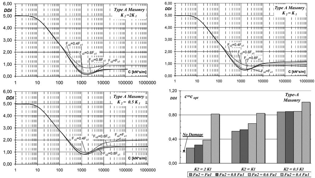
Figure 5. Type-A masonry: values of DDI as a function of viscous constant  $c$  (Calitri earthquake).
