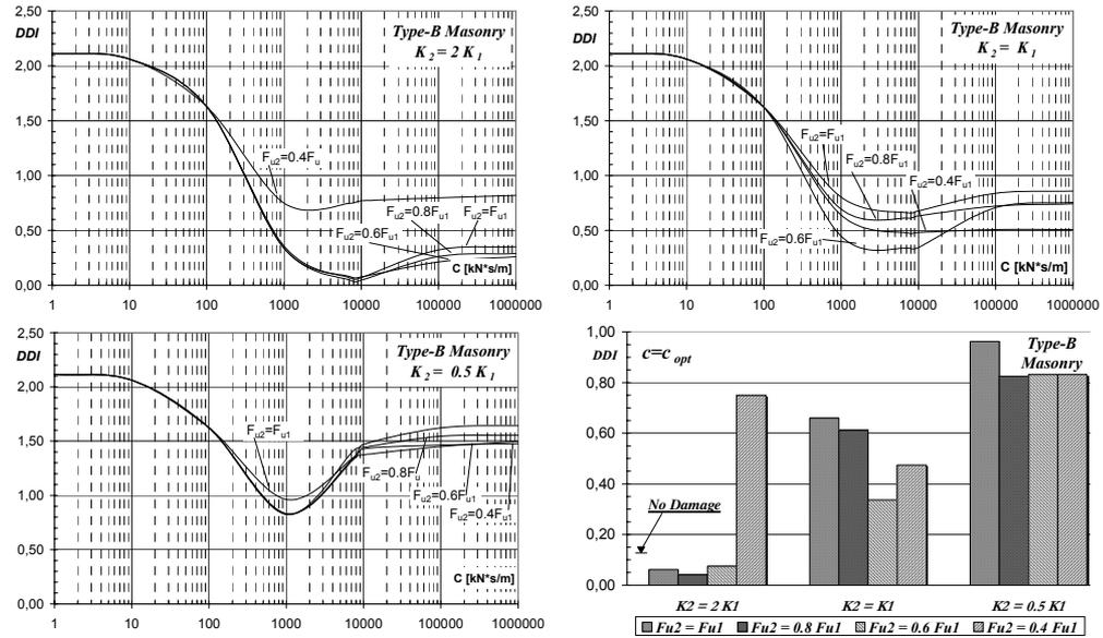
Figure 9. Type-B masonry: values of DDI as a function of viscous constant  $c$  (El Centro earthquake).
