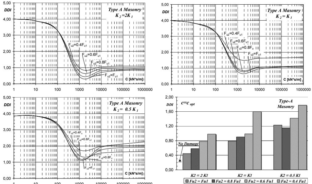
Figure 7. Type-A masonry: values of DDI as a function of viscous constant  $c$  (Taiwan earthquake).
