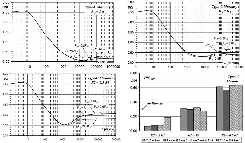
Figure 11. Type-C masonry: values of DDI as a function of viscous constant  $c$  (El Centro earthquake).
