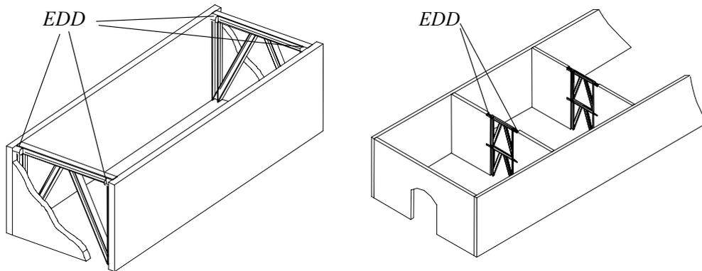
**Figure 2.** Possible locations of steel strengthening bracings and EDDs in masonry buildings
