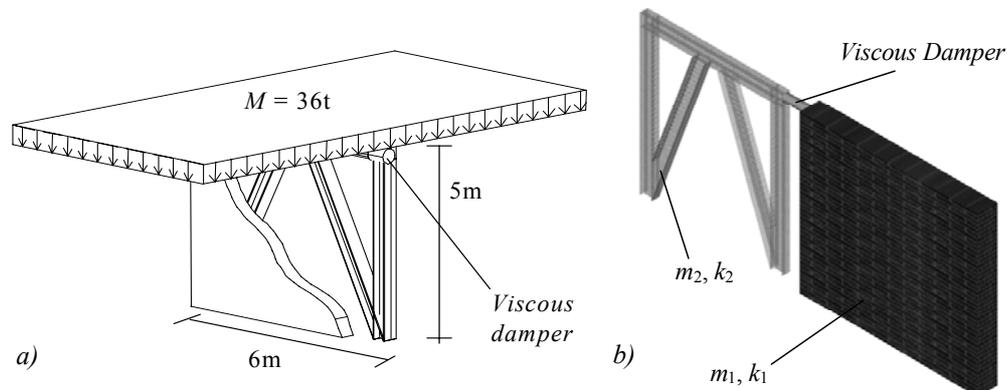
**Figure 1.** The model investigated in the analysis (a) and its plane schematization (b) .
