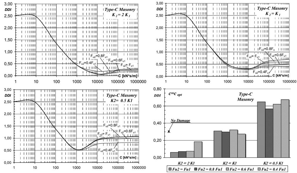
**Figure 12.** Type-C masonry: values of DDI as a function of viscous constant  $c$  (Taiwan earthquake).
