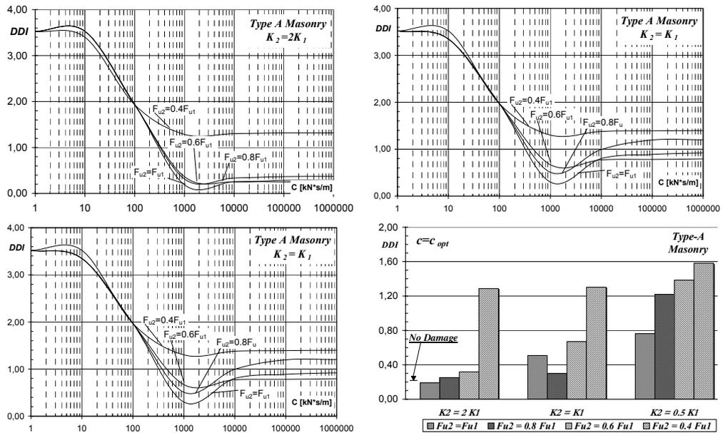
Figure 6. Type-A masonry: values of DDI as a function of viscous constant  $c$  (El Centro earthquake).
