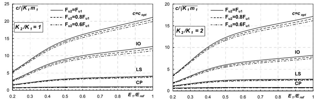
**Figure 13.** Nondimensional viscous constant for a given performance level versus  $E_1/E_{ref}$  ( $E_{ref} = 660 \text{ N/mm}^2$ ).
