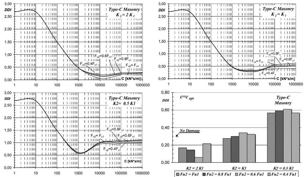
Figure 10. Type-C masonry: values of DDI as a function of viscous constant  $c$  (Calitri earthquake).
