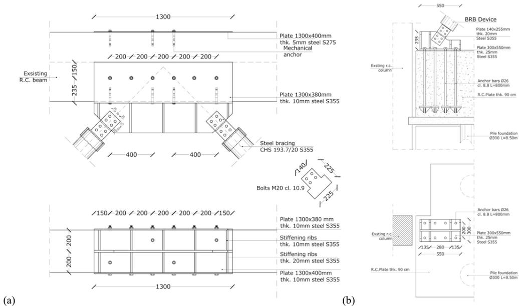
Fig. 9. (a) Connection of damped brace to RC beam; (b) Connection of damped brace to foundations.
