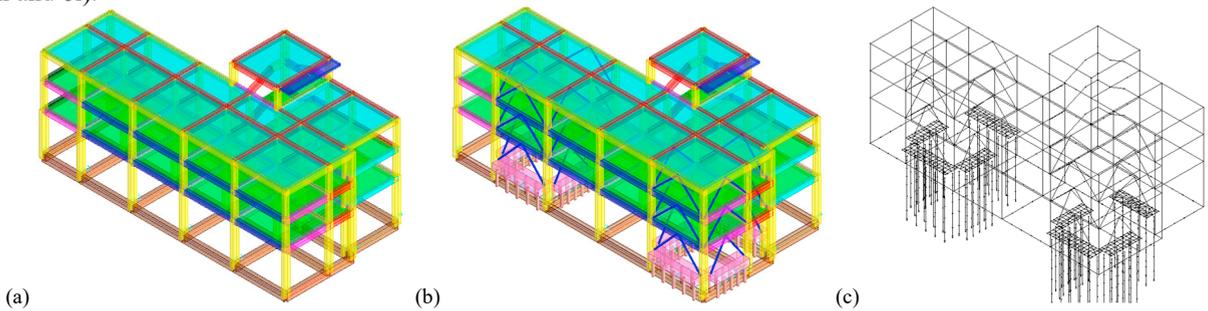
Fig. 4. (a) 3D view of the original building; (b) 3D view of the retrofitted building. (c) Fem model of the retrofitted building.
