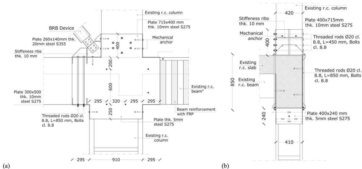
Fig. 10. Shear strengthening of beam-column joint with steel plates: (a) Front view; (b) Section view.
