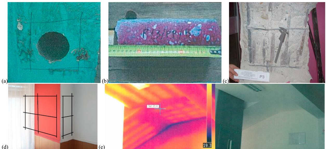
Fig. 3. (a) Coring of RC column; (b) Carbonation Depth Test; (c) Extraction of a steel bar sample from a column; (d) Pacometric test on a column to verify the positioning of steel bars; (e) Thermographic tests.
