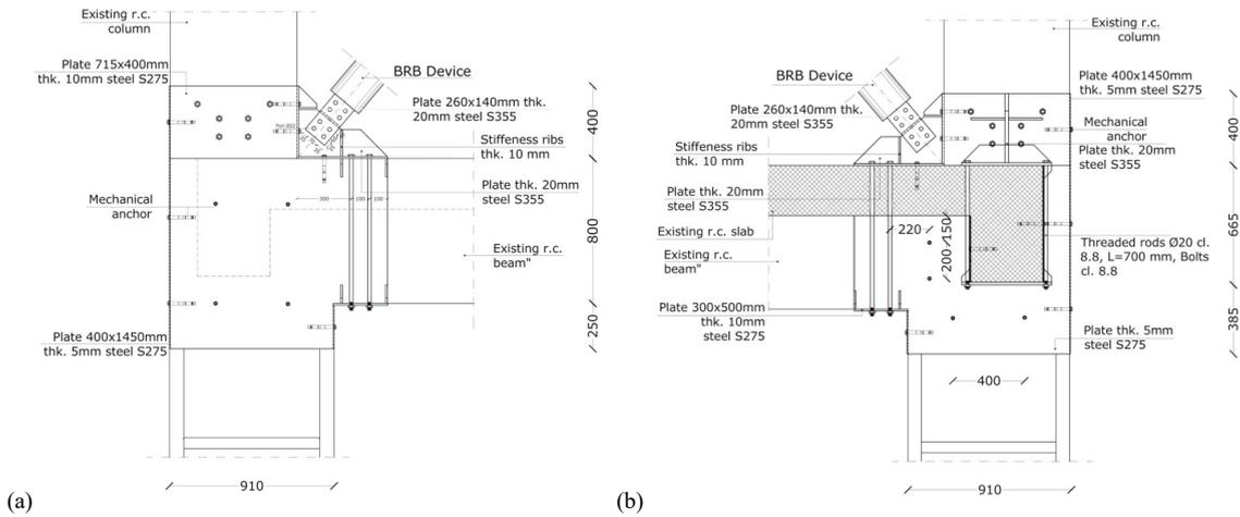
Fig. 8. (a) Connection of damped brace to column: (a) Front view; (b) Section view.
