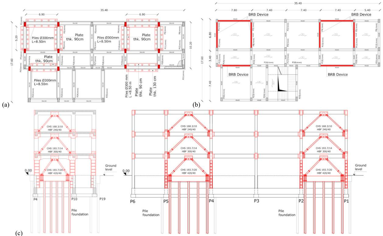
Fig. 5. (a) Retrofit of existing foundations; (b) Layout in plan of the damped braces; (c) Section views.
